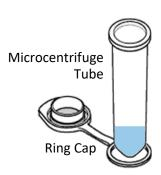
A Ring Cap is provided to conveniently store your sample in the Microcentrifuge Tube. Slide the Ring Cap on to the Microcentrifuge Tube from the bottom.
