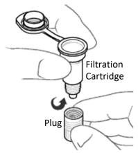
The Plug screws onto the base of the Filtration Cartridge. To ensure a tight seal, give a firm twist by hand.
