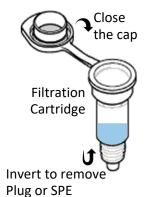
After sample and reagents have been added to the Filtration Cartridge, cap it and invert before unscrewing the Plug or OPTIONAL SPE Cartridge.
