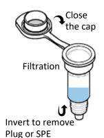
After sample and reagents have been added to the Filtration Cartridge, cap it and invert before unscrewing the Plug or SPE Cartridge.
